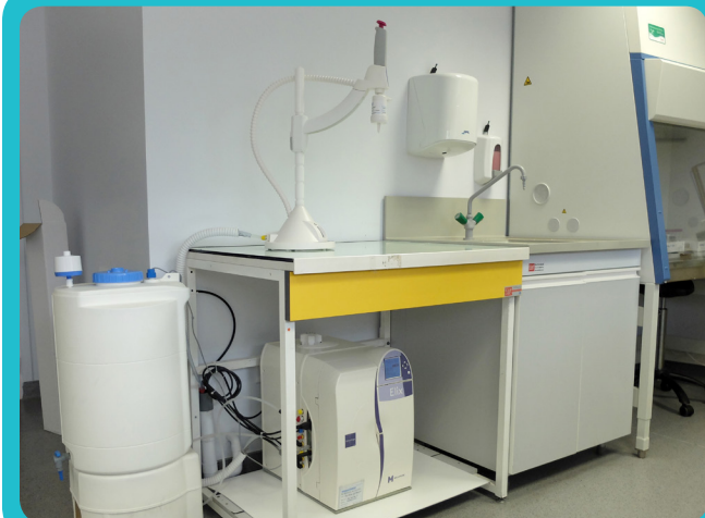
Elix® Advantage 3 system, E-POD® dispenser and a 60-liter storage tank in the Institute's histology laboratory.
