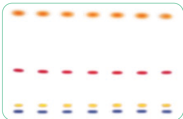
The chromatogram shows four clearly separated spots according to Ph. Eur. test conditions and fulfils Ph. Eur. requirements.
