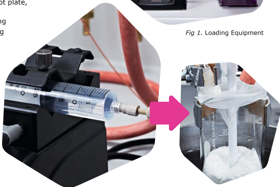
Fig 2. Concentrated API solution is added dropwise to a stirred and heated beaker containing Parateck SLC
