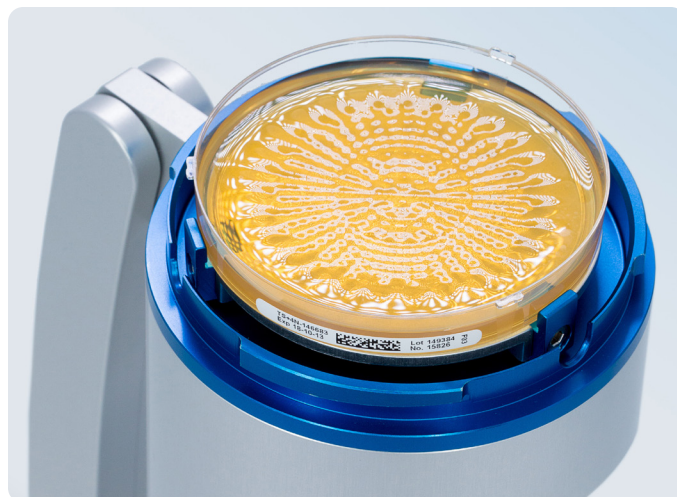
Figure 2: Standard 90 mm Petri dish on a MAS-100 NT® microbial air sampler. The impaction pattern generated by drawing 1000 l of air at 100 SLPM through a 300 x 0.6 mm perforated lid is clearly visible.
