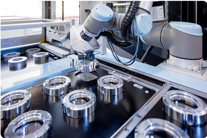
Figure 5: Perforated lids in production. Mounting robots in combination with the most modern machining tools produce parts within very narrow specifications.
