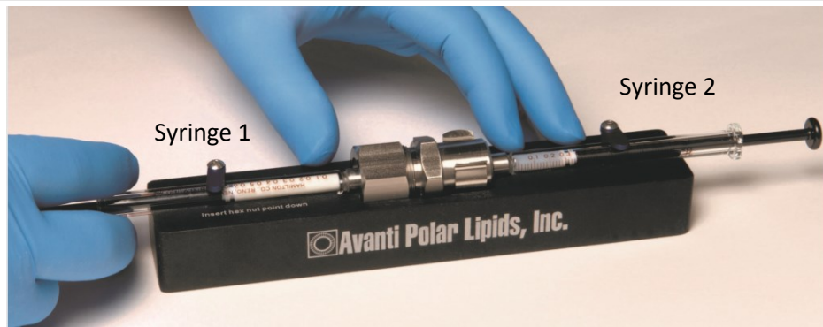
Figure 1: The lipid extrusion process. The MLV solution in Syringe 1 is transferred to Syringe 2 by gently pushing on the plunger of Syringe 1. The solution is then transferred back to Syringe 1 by gently pushing on the plunger of Syringe 2. This process is repeated for a total of 11 cycles.
